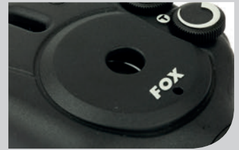
Cone speaker on MXr+ for enhanced sound quality
